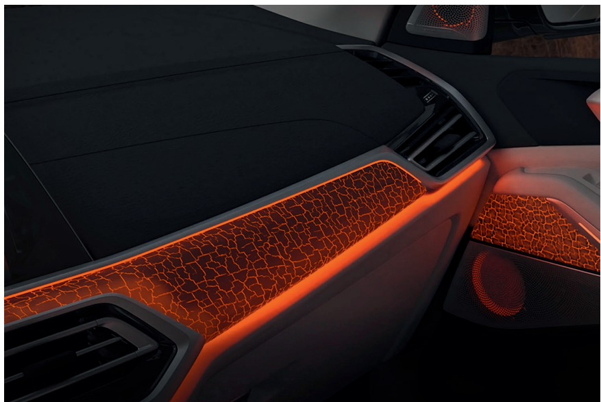
Decorative strips in the vehicle with partial transillumination in day-night design. © Reichle
